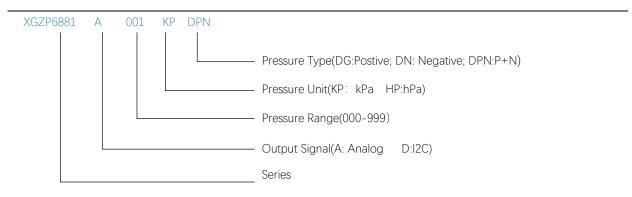
Note:1. Voltage 5Vdc as default value, add 33 behind mode signify 3.3V power supply, e.g. : XGZP6881A001KPDG33.2 Custom requirement or parameter, please consult CFSensor for custom code(e.g custom pressure range etc.,)
