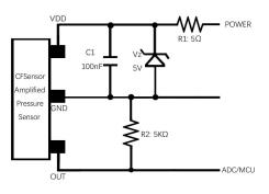
Note: Diagram state schematic connection only; Check Pin allocation in Dimension drawing.
